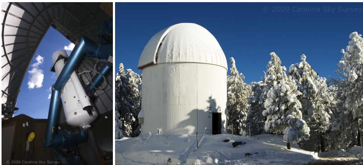
Figure 1 – The Catalina Sky Survey Schmidt telescope on Mount Bigelow, MPC code 703. This is the configuration of the telescope when configured with its 4K CCD camera.
