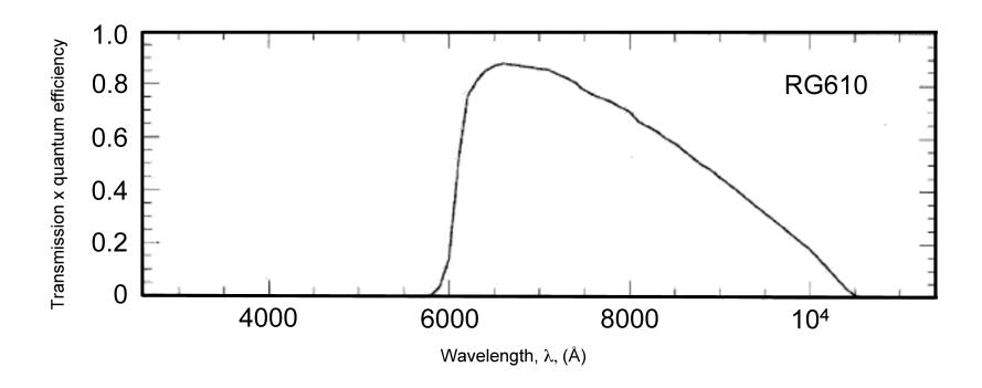
The characteristics of the red, RG610 filter and QUEST camera used by NEAT in the point-and-shoot mode as published by Baltay et al.
