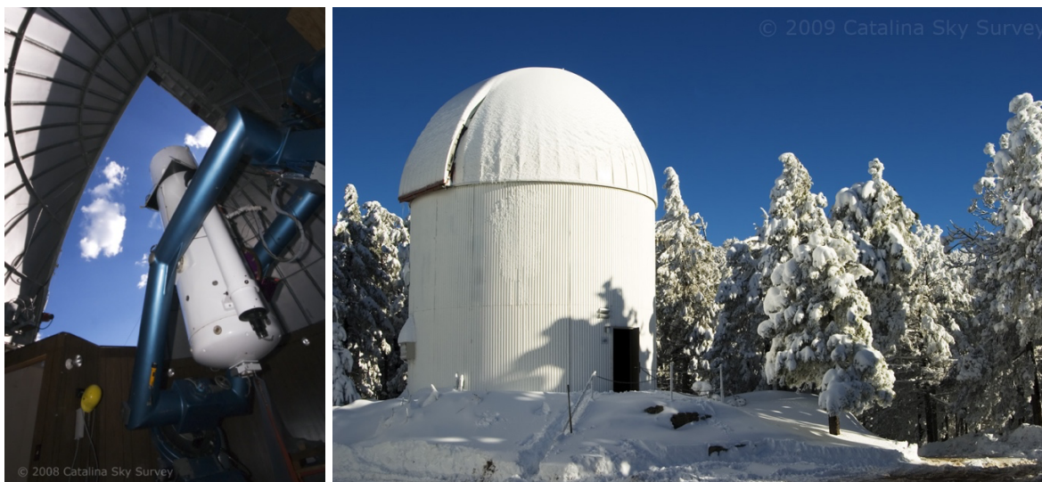
Figure 1 – The Catalina Sky Survey Schmidt telescope on Mount Bigelow, MPC code 703. This is the configuration of the telescope with its 4K x 4K CCD camera between 2003-2016. Catalina Sky Survey, L: 2008, R: 2009
