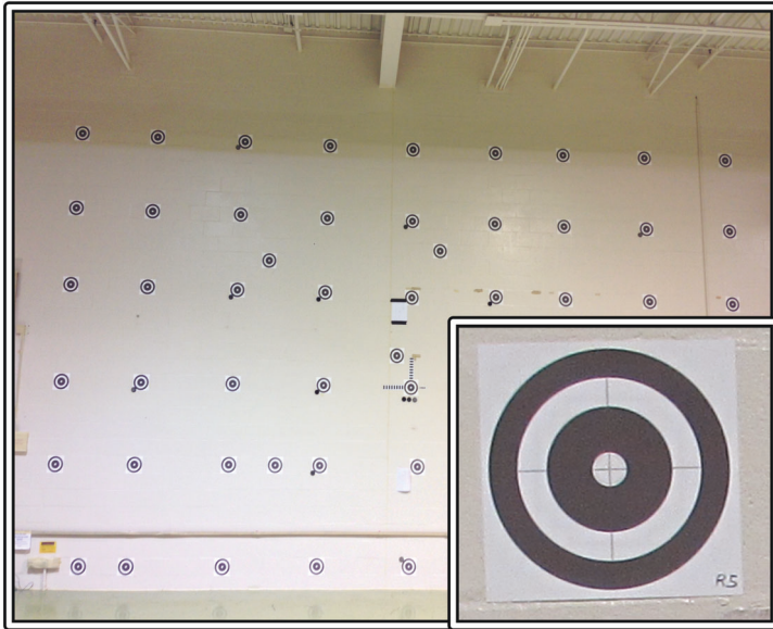
Fig. 10 The OLA calibration wall is shown. An individual target is shown in the inset
