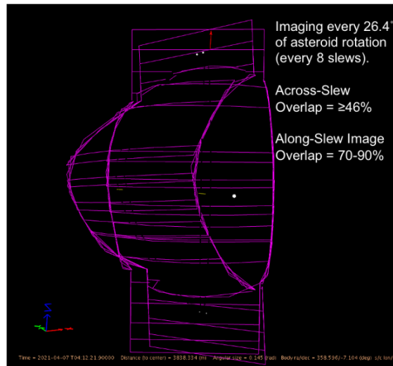
Figure 5 MapCam footprints demonstrating along-slew overlap and across-slew overlap.
