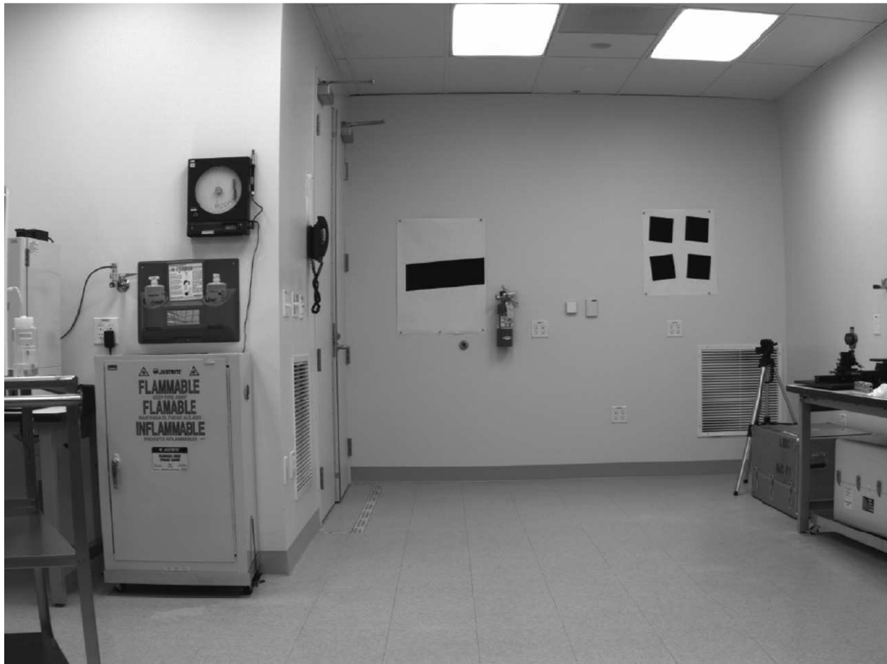
Figure 7. NavCam 1 image of an optical target located 8 m away at Malin Space Science Systems, illustrating the NavCam image quality at the required object distance.
