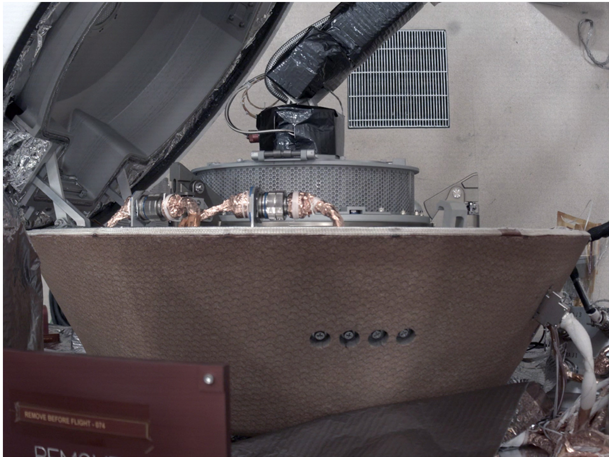
Figure 18. StowCam image taken during ground testing showing the TAGSAM sampler head latched into the SRC capture ring
