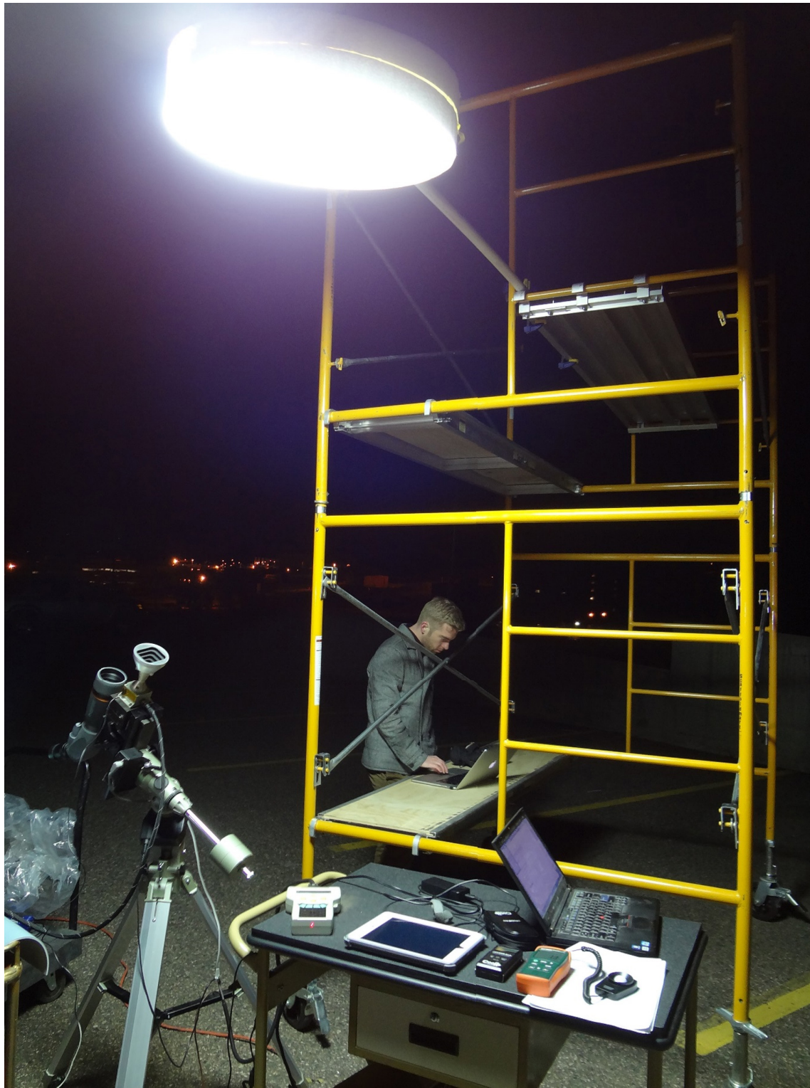
Figure 14. EM NavCam night sky imaging test setup with simulated asteroid in the field of view. The EM NavCam is mounted to a motorized tripod with an integral star finder.
