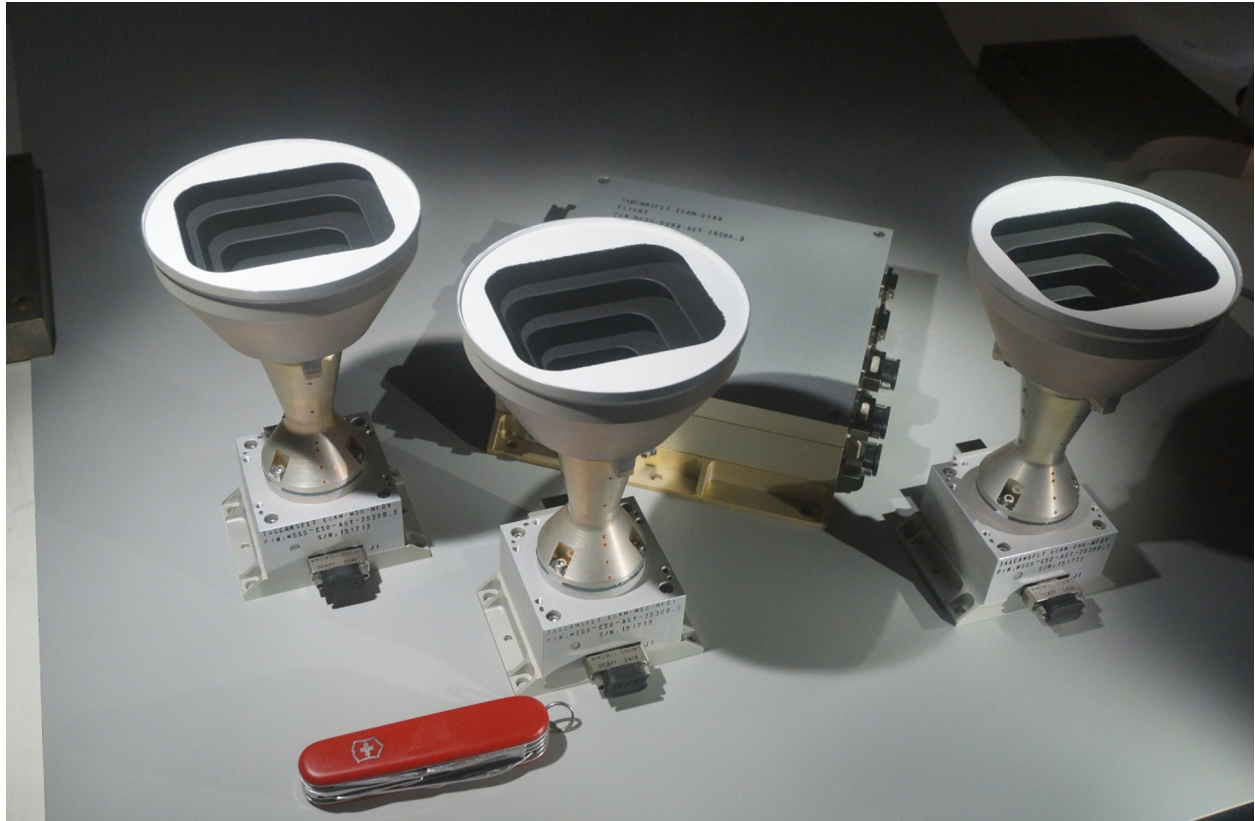
Figure 1. Flight TAGCAMS camera heads and DVR, shown with the 84 mm long pocketknife for scale. The two DVRs are shown stacked on top of each other.
