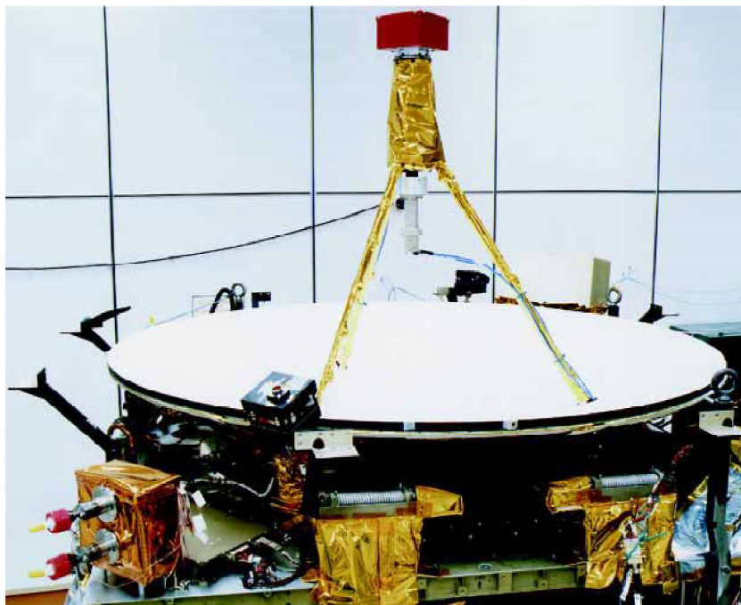
Figure 1. The NEAR Magnetic Field Instrument. The sensor for the instrument is mounted inside the tube covered with gold foil, just below the red box at the top of the antenna feed for NEAR's telemetry antenna.
