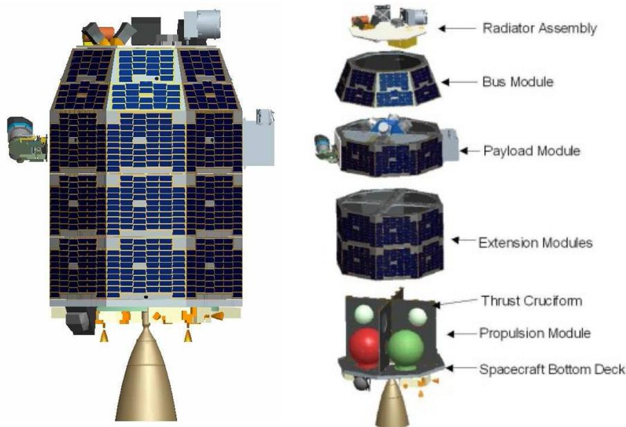
Figure 3-1: LADEE major structural components and layout
