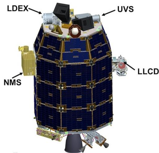
**Figure 1-1: The LADEE Spacecraft and Instrument Locations**
