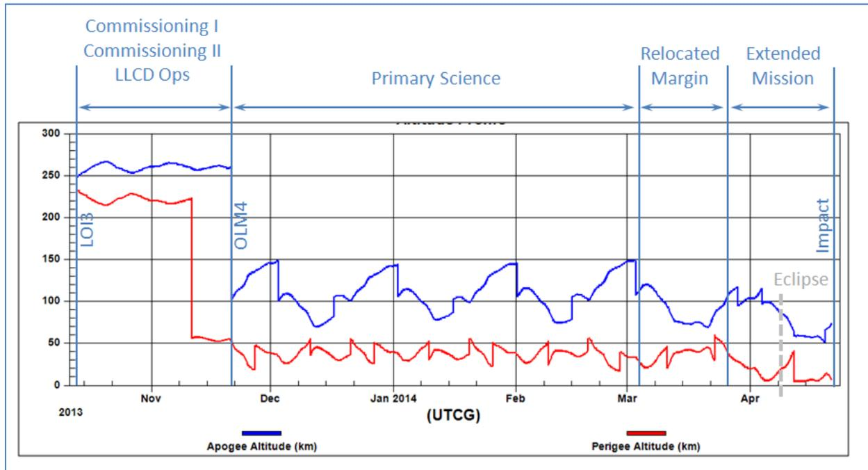
**Figure 4-3: LADEE orbit altitude profile throughout the commissioning, science, and extended science mission phases. Note the extended science phase covered the relocated margin + extended mission intervals.**
