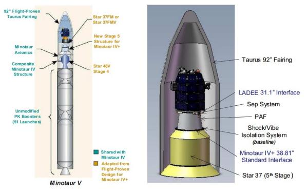
Figure 2-1: LADEE launch vehicle and configuration
