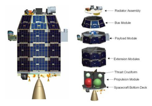
Figure 3-1: LADEE major structural components and layout
