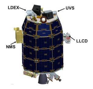
Figure 3-1: The LADEE Spacecraft and Instrument Locations
