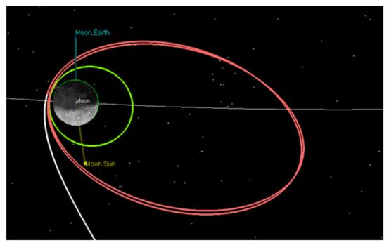
Figure 4-2: LOI phase of the LADEE mission. Last phasing loop (white), LOI-1 orbits (orange), LOI-2 orbits (green), and LOI-3 transition to the commissioning orbit (darker green semi-circle on the upper half of the Moon)
