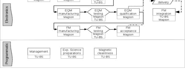
Fiaure 7: The MAG instrument work flow loaic with task and responsible body identification.
