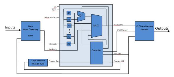
The processor was originally developed for the NASA Themis mission and it has since then continuously been improved and expanded in its functionality. It is used successfully for the Themis mission as well as in reaction wheels, attitude control magnetometers, magneto-torquers and other terrestrial applications and will also be used for the MPO and MMO magnetometers of the ESA/JAXA BepiColombo mission
