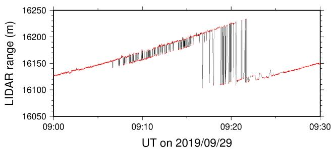
Figure 3. An example of saw-toothed LIDAR range profile.
