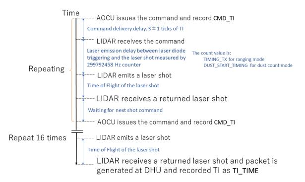
Figure 1 Timing chart of the laser shot events and recorded variables for ranging mode and dust count mode. The INTERVAL value is set to 1 is assumed for the ranging mode in this figure.
