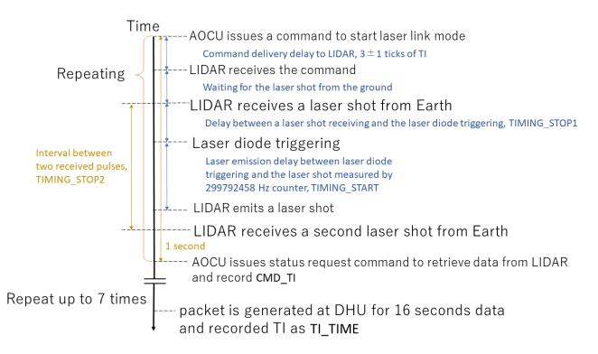
Figure 2 Timing chart of the laser shot events and recorded variables for laser link mode.
