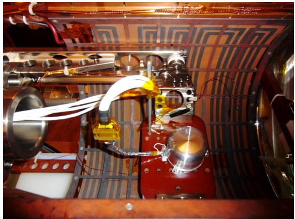
Fig. 4 The MasMag sensor placed within the temperature chamber on a rotational platform for calibrations in the Magnetsrode facility
