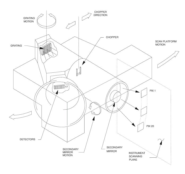
Fig. 2. Schematic Diagram of the Instrument and Scanning Motions.
