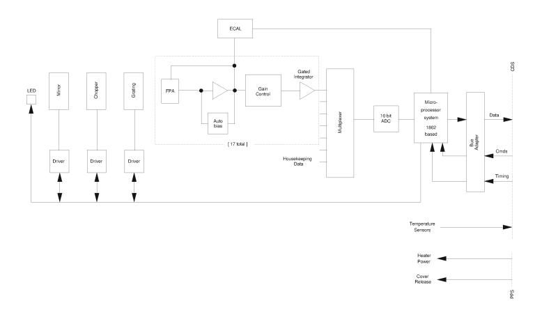
Fig. 7. Electronics Block Diagram.
