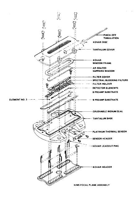
Fig. 5. Focal Plane Assembly Components.
