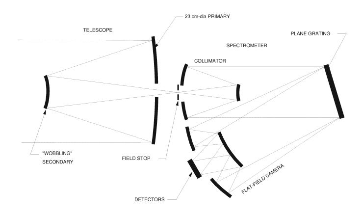
Fig. 3. Schematic of the NIMS Optical Design.
