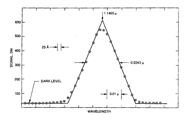
Fig. 11. Spectral Bandpass Response.
