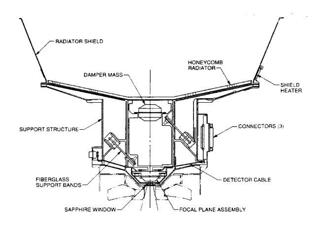
Fig. 6. Radiative Cooler Assembly.
