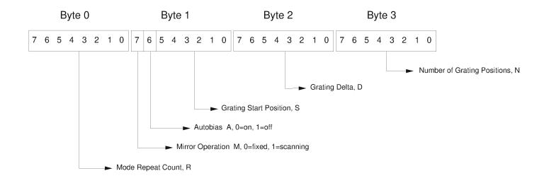
Fig. 13. Parameter Table Assignments.
