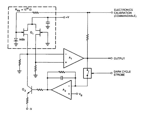
Fig. 8. Preamplifier and Autobias Circuitry.
