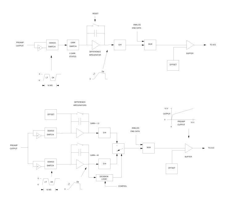
Fig. 9. Analog Signal Chain Electronics.
