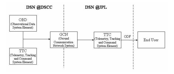
Figure 2-1. Data Flow for Orbit Data File Interface
