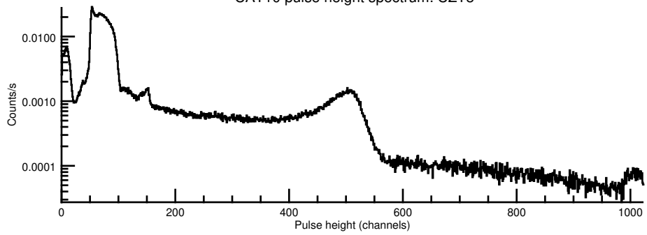
CAT10 pulse height spectrum: CZT3
