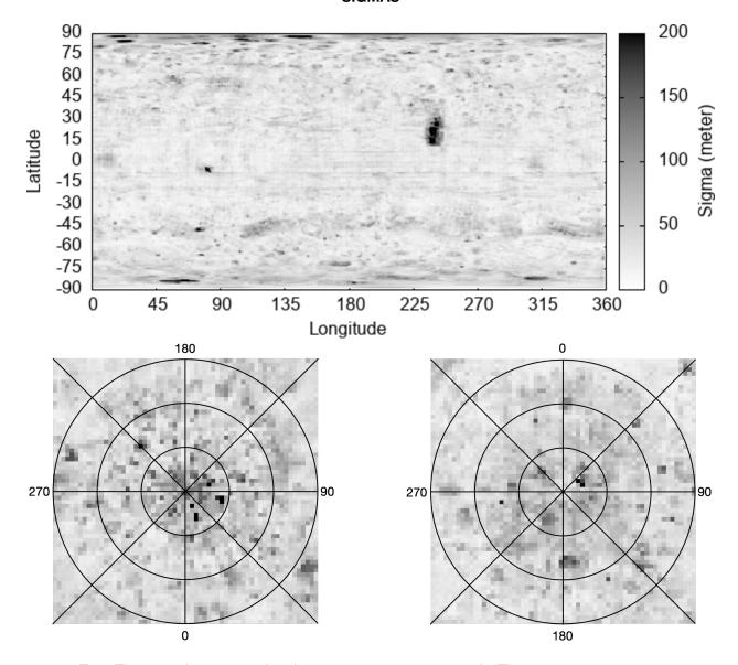
Top: This panel presents the data in ceres\_sigmas\_c.cub. The worst sigma is ~570 m, which is less than half the GSD of the Q=512 model, indicating the maplets agree to a high confidence level. Sigmas of ~250 m occur near the poles where there is a smaller range of sun angles. Sigmas everywhere are good for the global model, hence the reasons for higher sigmas in various regions are outside the scope of this project.
