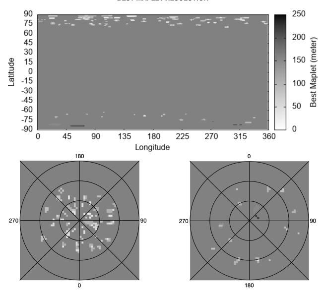
Top: This panel presents the data in ceres\_bestmap\_c.cub. Most of Ceres is covered by maplets with a GSD of 160 m. Craters near the poles have higher resolution maplets, reaching to 16 m in some places, though a few bins at the south pole have maplets with a GSD of 250 m. The best maplet resolution is much greater than the global model, giving confidence to the global model uncertainties.
