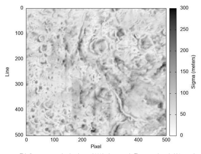
This figure presents the data in teqn01113\_sigma\_c.cub. The worst sigma is 291 m and the best sigma is ~1 m, with the average sigma ~81 m. Since the worst sigma is less than the regional DTM GSD (360 m/vertex), the sigmas are quite good. **As such, the reasons for higher sigmas in various regions are outside the scope of this project.**
