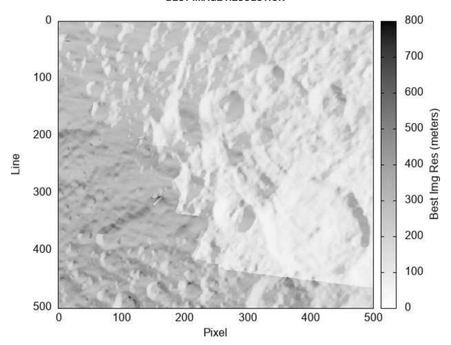
This figure presents the same information as teqn01113\_bestimg\_c.cub. The worst image resolution is ~800 m/px and the best images resolution is ~45 m/px. About 91% of the regional DTM (with a GSD of 360 m/vertex) under samples the best image resolution, and in these areas the effective resolution is that of the regional DTM GSD. The rest of the regional DTM over samples the best image resolution, and in those areas the effective resolution is limited by that of the best image resolution.
