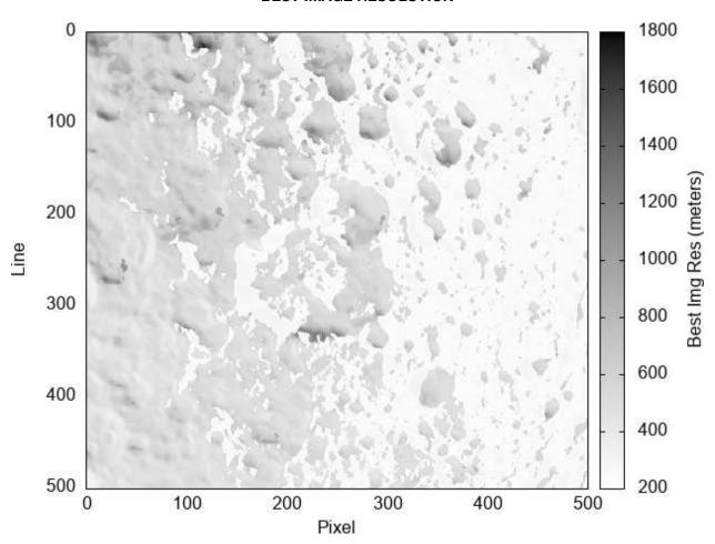
This figure presents the same information as thln48083\_bestimg\_c.cub. The worst image resolution is  $\sim$ 1725 m/px and the best is  $\sim$ 235 m/px. About 46% of the regional DTM (with a GSD of 400 m/vertex) under samples the best image resolution, and in these areas the effective resolution is that of the regional DTM GSD. The rest of the regional DTM over samples the best image resolution, and in those areas the effective resolution is limited by that of the best image resolution.
