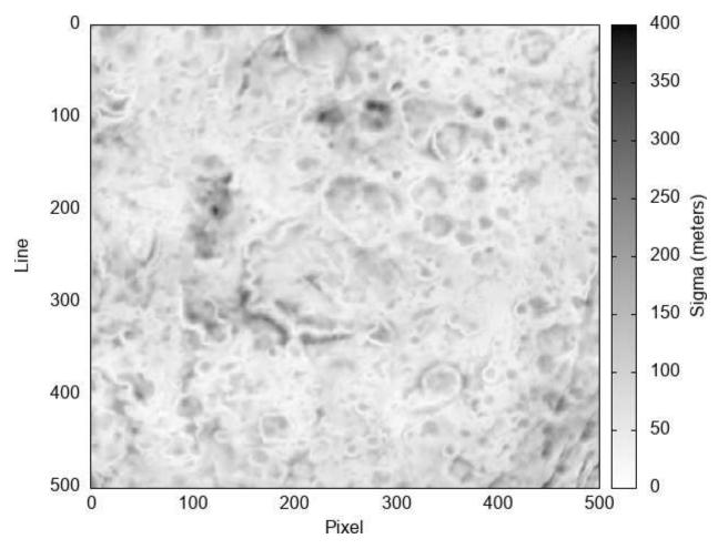
This figure presents the data in thln48083\_sigma\_c.cub. The worst sigma is 357 m and the best sigma is ~1 m, with the average sigma ~82 m. Since the worst sigma is less than the regional DTM GSD (400 m/vertex), the sigmas are quite good. **As such, the reasons for higher sigmas in various regions are outside the scope of this project.**
