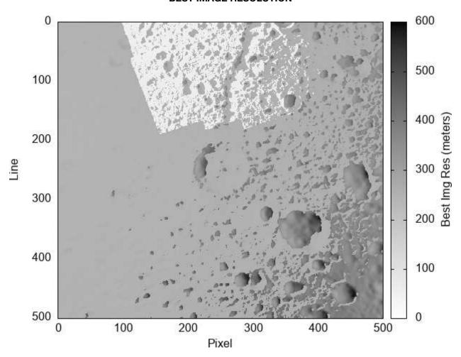
This figure presents the same information as leqs00294\_bestimg\_c.cub. The worst image resolution is  $\sim$ 594 m/px and the best is  $\sim$ 50 m/px. About 96% of the regional DTM (with a GSD of 405 m/vertex) under samples the best image resolution, and in these areas the effective resolution is that of the regional DTM GSD. The rest of the regional DTM over samples the best image resolution, and in those areas the effective resolution is limited by that of the best image resolution.
