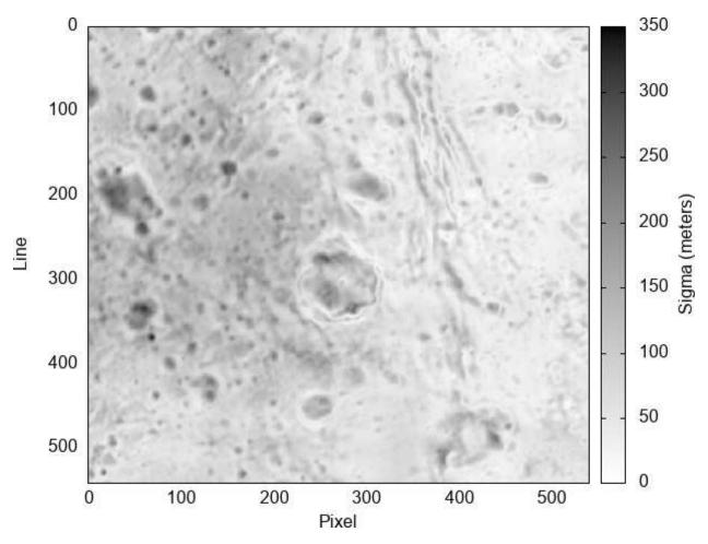
This figure presents the same information as lhln50284\_sigma\_c.cub. The worst sigma is 334 m and the best sigma is ~1 m, with the average sigma ~85 m. Since the sigmas are everywhere less than the regional DTM GSD (370 m/vertex), the sigmas are not large enough to worsen the effective resolution of the topography. As such, the reasons for higher sigmas in various regions are outside the scope of this project.
