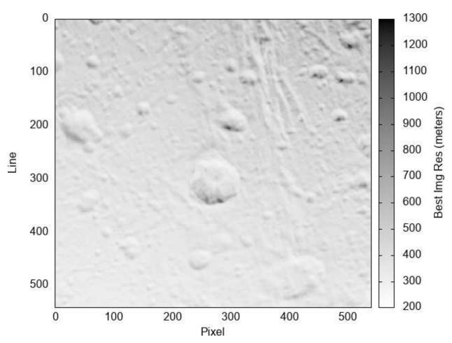
This figure presents the same information as lhln50284\_bestimg\_c.cub. The worst image resolution is ~1242 m/px and the best is ~269 m/px. About 31% of the regional DTM (with a GSD of 370 m/vertex) under samples the best image resolution, and in these areas the effective resolution is that of the regional DTM GSD. The rest of the regional DTM over samples the best image resolution, and hence the effective resolution is usually limited by that of the best image resolution.
