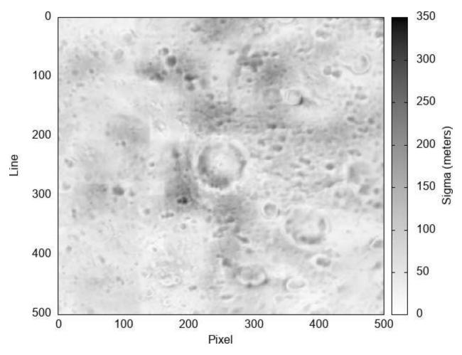
This figure presents the data in leqs00294\_sigma\_c.cub. The worst sigma is 314 m and the best sigma is ~1 m, with the average sigma ~82 m. Since the sigmas are everywhere less than twice that of the regional DTM GSD (405 m/vertex), the sigmas are not large enough to worsen the effective resolution of the topography. As such, the reasons for higher sigmas in various regions are outside the scope of this project.
