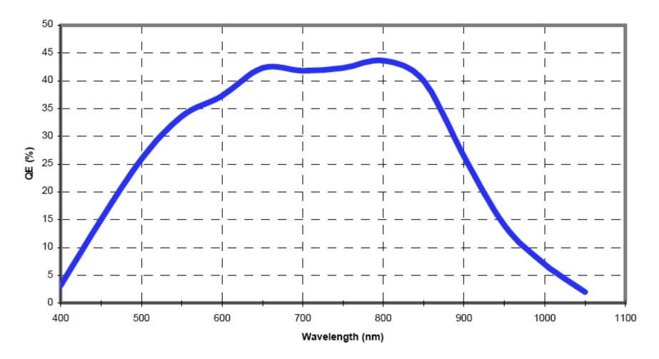
The quantum efficiency for the Fairchild CCD485 chip. These chips are used by NEAT Palomar tri-camera and the camera used at the Mt. Haleakala, Maui site.
