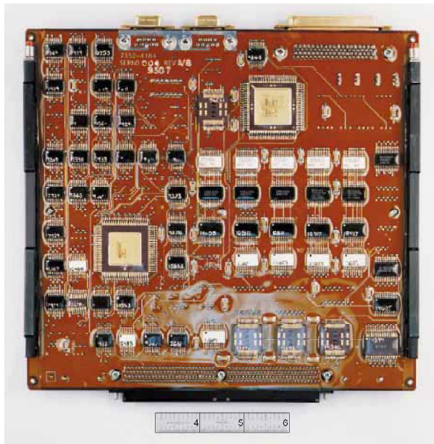
Figure 4. (a) Top and (b) bottom views of the RTX2010 processor board removed from the command and telemetry processor chassis (scale is in inches).
