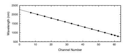
Figure 5: Spectral calibration data and linear regression.
