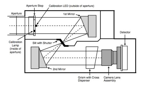
Figure 1: Schematic optical design of the NIRS.
