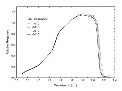
Figure 3: Spectral responsivity of InGaAs detector array depending on temperature.
