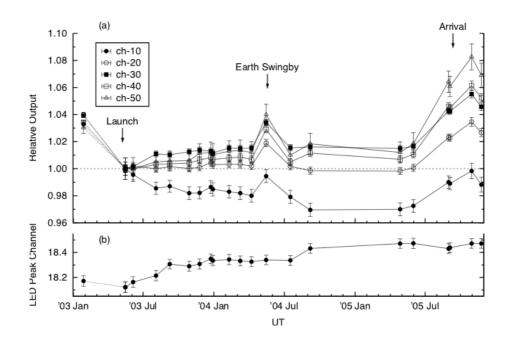
**Figure 7:** Time series plots for (a) the NIRS channel responses in lamp observation and (b) the peak channels in LED observation.
