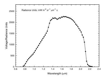
**Figure 6:** The radiometric calibration of the NIRS determined from laboratory tests, corresponding to a field filling source.
