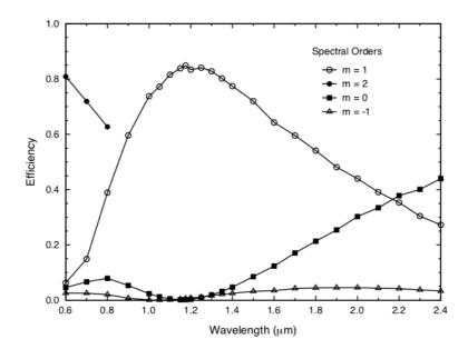
**Figure 4:** The measured grism efficiency for different spectral orders.
