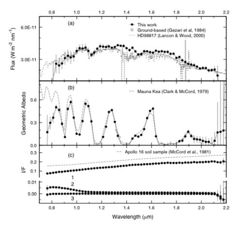
**Figure 8:** Representative NIRS spectra obtained from in-flgith measurements: (a) Antares, (b) Jupiter, (c) Moon. The spectra used for comparison were taken by the ground-based telescopes (Lancon and Wood, 2000; Clark and McCord, 1979).
