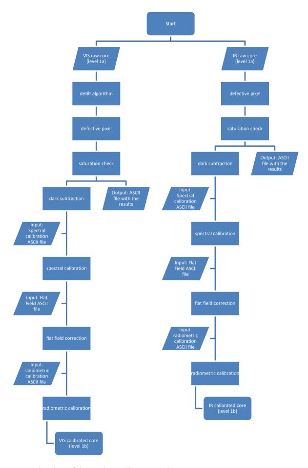
Figure 4. Flowchart of the VIR data calibration pipeline
