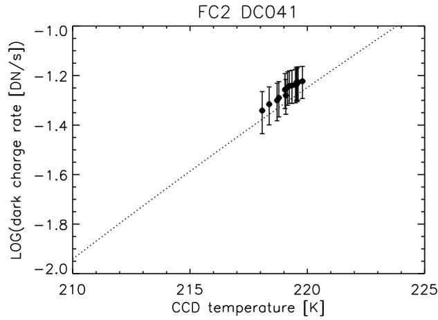
**Figure 2: FC2 bulk dark current for DC041**
