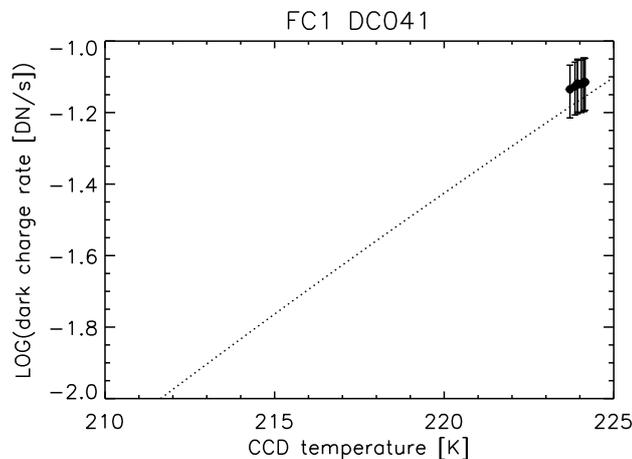
Figure 1: FC1 bulk dark current for DC041
