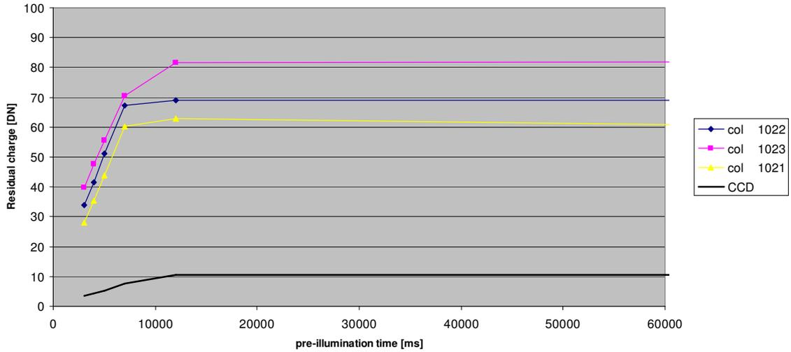
Figure 7: FC1 extra charge levels in DC041
