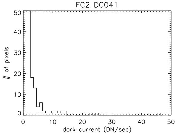
**Figure 5: FC2 hot pixel histogram in DC041**
