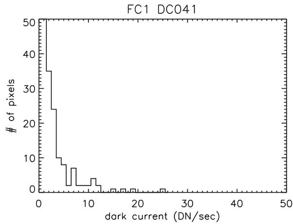
**Figure 3: FC1 warm pixel histogram in DC041**
