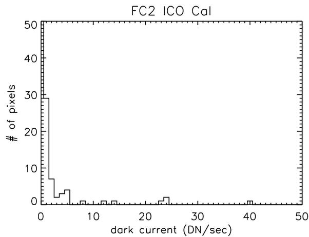
**Figure 6: FC2 hot pixel histogram in ICO**
