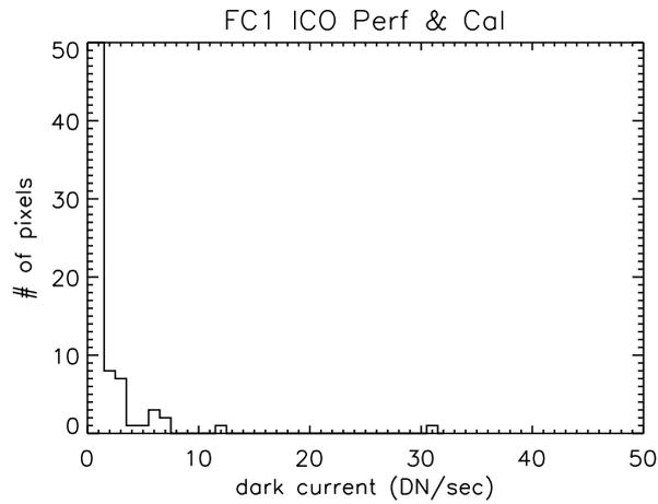
**Figure 4: FC1 warm pixel histogram in ICO**
