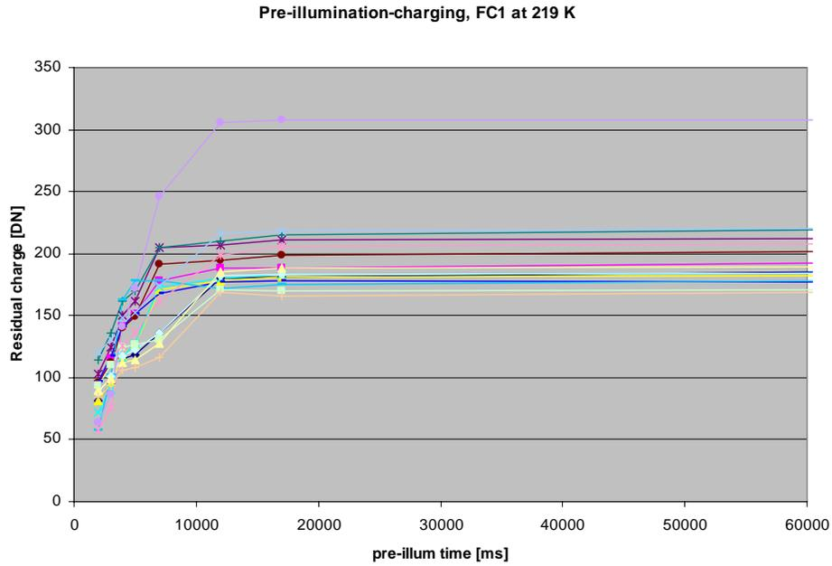
Figure 16. Extra charge on the FC1 CCD during ICO CCDcal at 219 K (16 highest pixels of column 1024).
