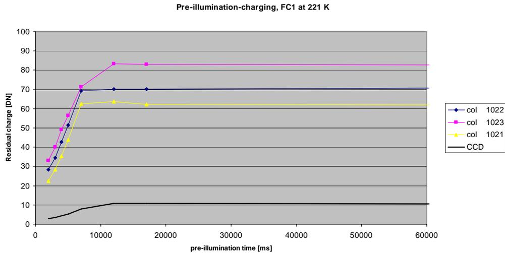
Figure 19. Average extra charge (columns and whole CCD) for FC1 during ICO Calibration at 221 K.
