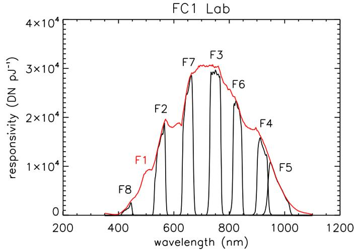
**Figure 8.** The absolute responsivity of the FC1 through the different color filters as determined from the lab calibration. Note that the responsivity determined from flight data is larger!
