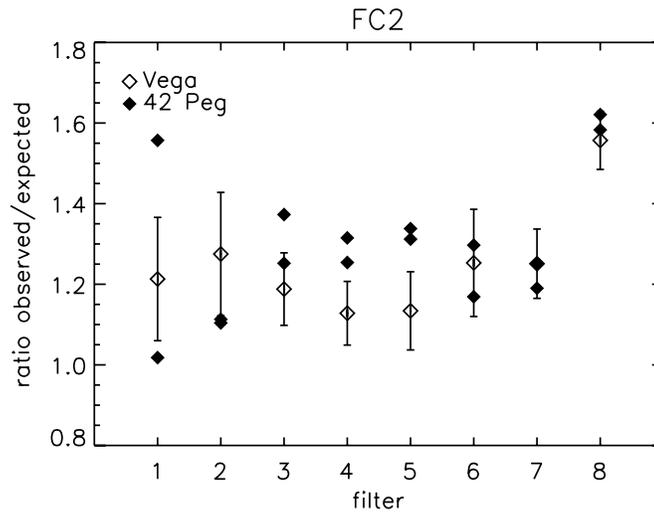
**Figure 12.** The stellar flux observed by FC2 in the different filters compared to that expected from the laboratory calibration of FC1. The Vega data are mean and standard deviation of ~10 observations. The 42 Peg data are two single observations per filter.
