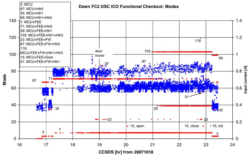
Figure 22 Variation of key value and input current for FC2 ICO Functional test
