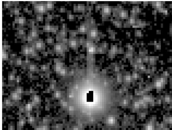
**Figure 13.** Charge blooming upward of an overexposed star in the 20 Cep starfield (from a FC2 600 sec clear filter exposure in the Performance block). The overexposed pixels at the center of the stars are marked in black.
