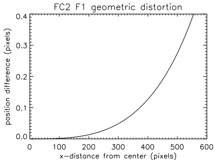
**Figure 6.** Geometric distortion of images taken through the clear filter (F1) of FC2 as determined from a fit of the radial distortion model to 36 star positions.
