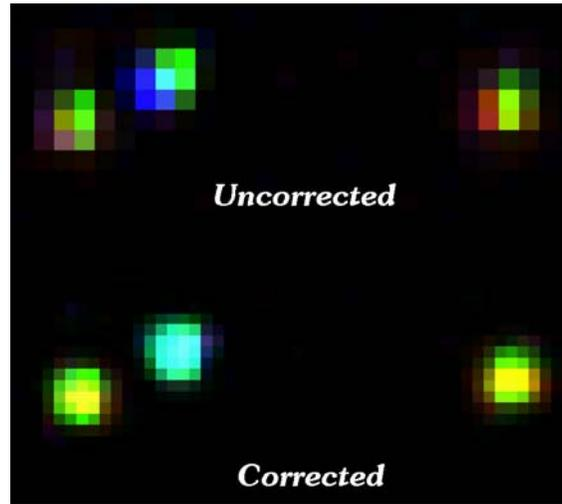
**Figure 7.** Star images taken through the different color filters need to be corrected for geometric distortion before combining them into a single color image. Here, both frames show a color composite of the same three stars, with (bottom) and without (top) prior geometric correction.
