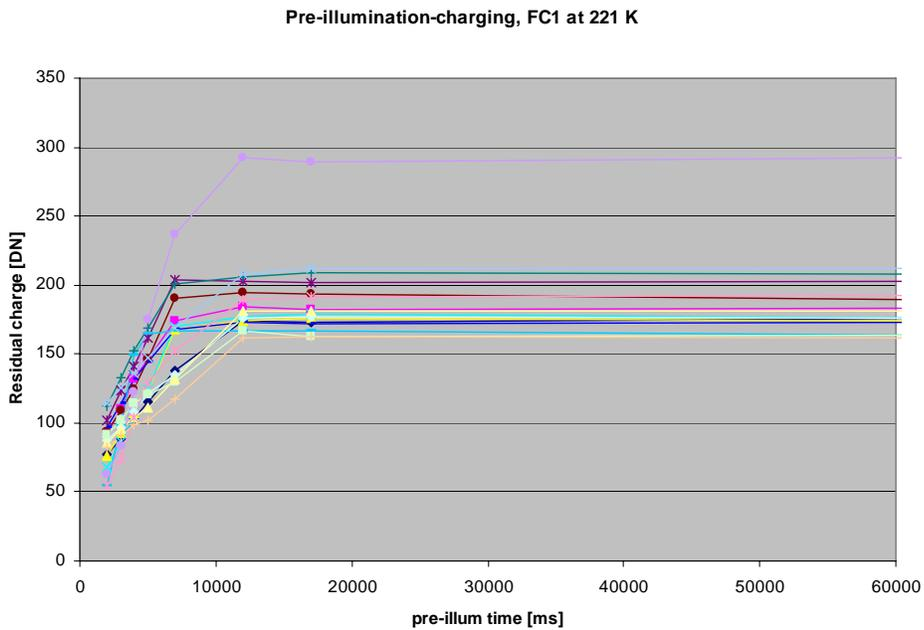
Figure 17. Extra charge on the FC1 CCD during ICO Calibration at 221 K (16 highest pixels of column 1024).
