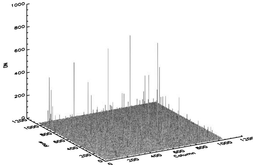
**Figure 1.** Dark current accumulated by the FC2 CCD in 300 sec (Performance block). The figure has been capped at 1000 DN, but there are 10 pixels exceeding this value.
