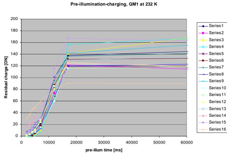
Figure 14. Extra charge on the QM1 CCD. Shown are the 16 most affected pixels per column at 232 K.
