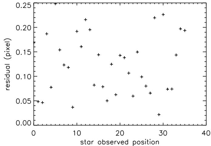
**Figure 5.** Typical residuals of the FC radial distortion model, i.e. the difference of a star's observed position in the geometrically corrected image (estimated from a 2D Gaussian fit to the brightness profile) and that expected from its sky coordinates ( $n = 36$ ).
