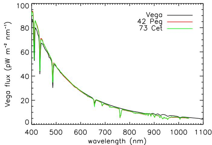
**Figure 9.** The spectrum of the three stars that were observed during ICO. The fluxes of 73 Cet and 42 Peg were equalized to that of Vega at 500 nm (by multiplying by 51.06 and 22.93, respectively). Spectral types are Vega: A0V, 73 Cet: B9III, and 42 Peg: B8V.
