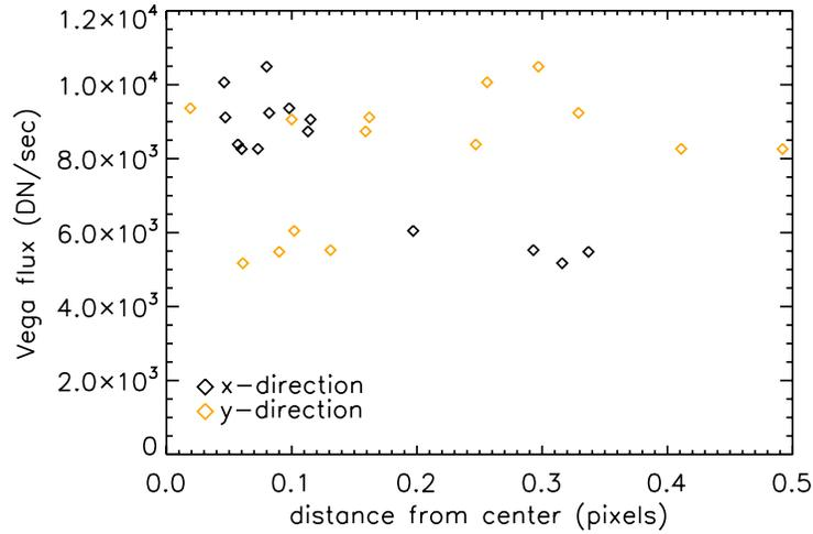
**Figure 10.** The measured stellar flux depends strongly on the position of the PSF on the pixel, especially in x-direction because of the presence of anti-blooming gates. The x-axis denotes the distance of the center of the PSF to the center of a pixel, as determined by a 2D Gaussian fit.
