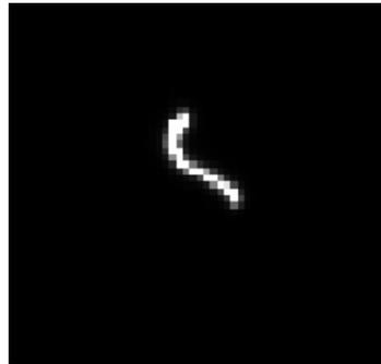
**Figure 4.** S/C jitter during Vega slew (60sec exposure time).
