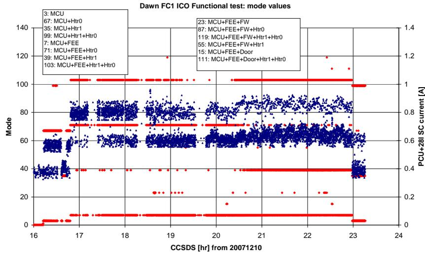
Figure 21 Variation of key value and input current for FC1 ICO Functional test
