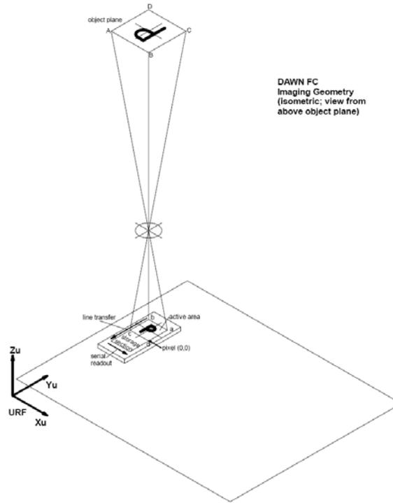
**Figure 29.** FC imaging geometry and coordinate system.
