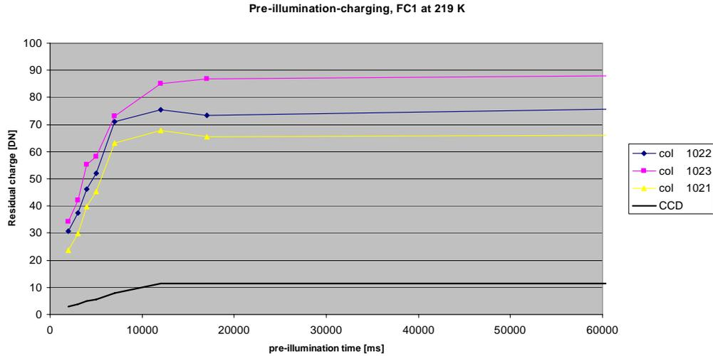
Figure 18: Average extra charge (columns and whole CCD) for FC1 during ICO CCDcal at 219 K.
