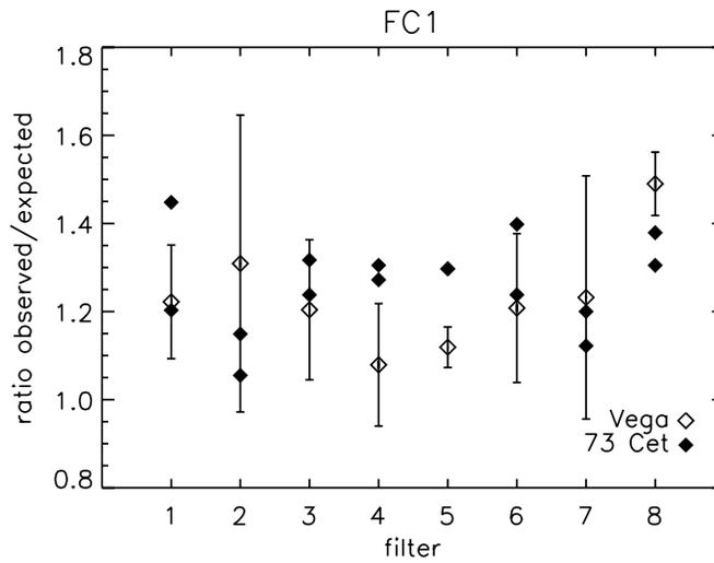
**Figure 11.** The stellar flux observed by FC1 in the different filters compared to that expected from the laboratory calibration. The Vega data are mean and standard deviation of ~10 observations. The 73 Cet data are two single observations per filter.
