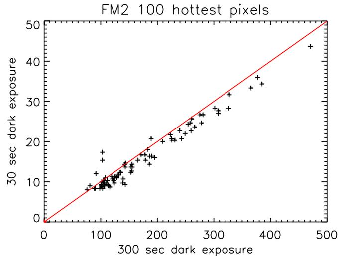
**Figure 2.** Dark current of the FC2 (FM2) CCD from the Calibration block data. We compare the charge acquired by the 100 hottest pixels in the active area in 300 sec to that in 30 sec. The dark current increases approximately linear with time, within the uncertainty imposed by the bias (~1 DN).
