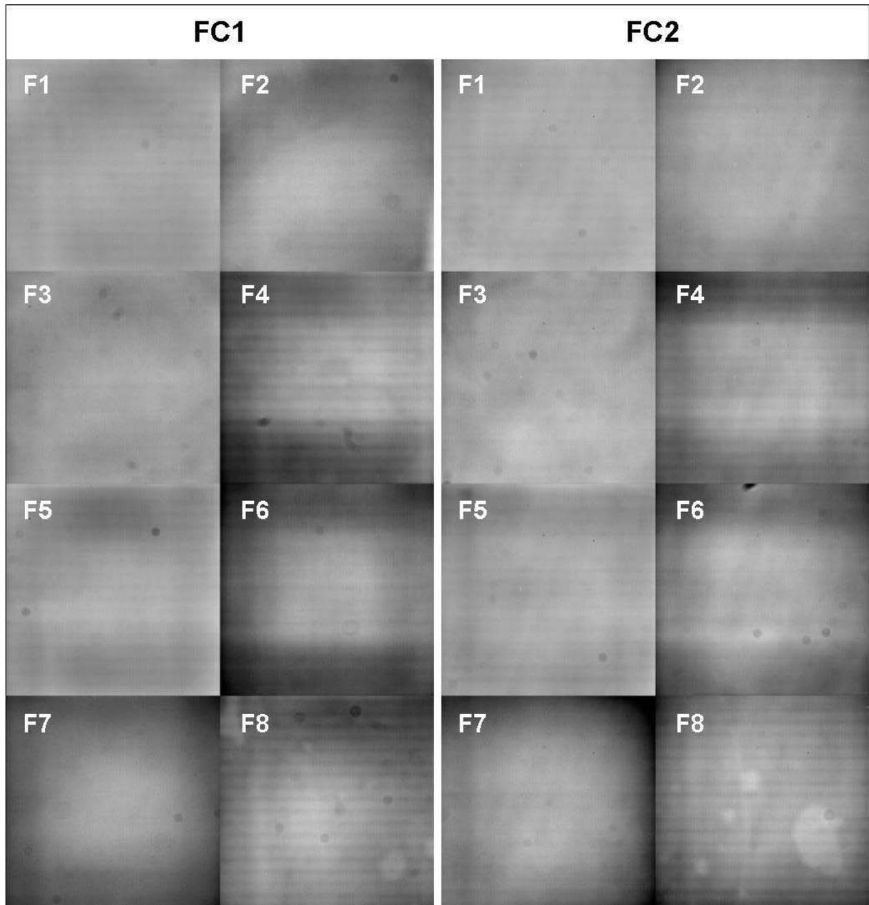
Figure 6. The normalized flat fields of FC1 (left) and FC2 (right). Brightness is scaled such that values  $<0.90$  are displayed as black, and values  $>1.05$  as white. A faint diagonal pattern is due to stray light associated with the experimental setup.
