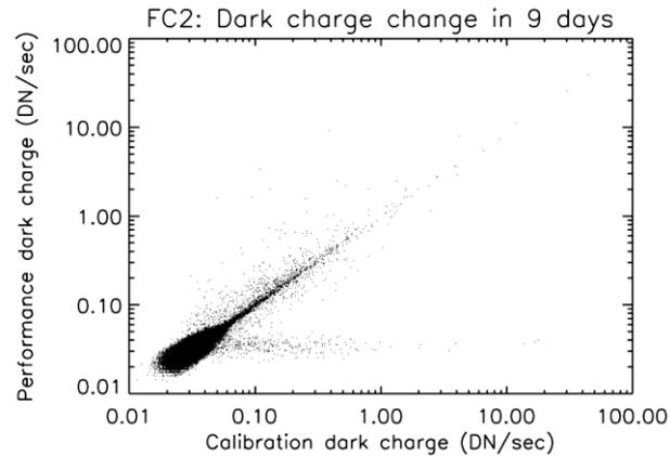
**Figure 4. FC2 dark current evolution over the course of the 9 days from the *ICO Performance* to the *Calibration* blocks . New warm pixels are located in the horizontal branch at the bottom.**
