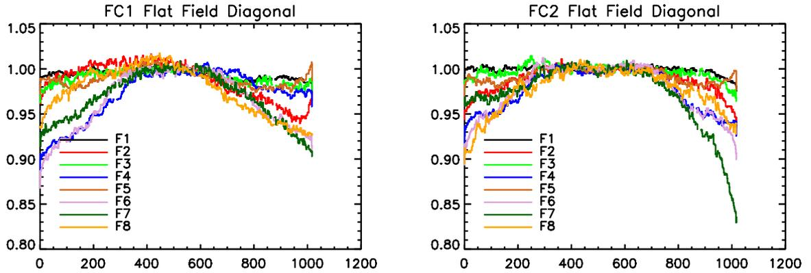
Figure 7. Diagonal profiles through the flat fields in Figure 6, running from pixel [0,0] to [1023,1023]. The profiles have been subjected to a 7-pixel wide median filter.
