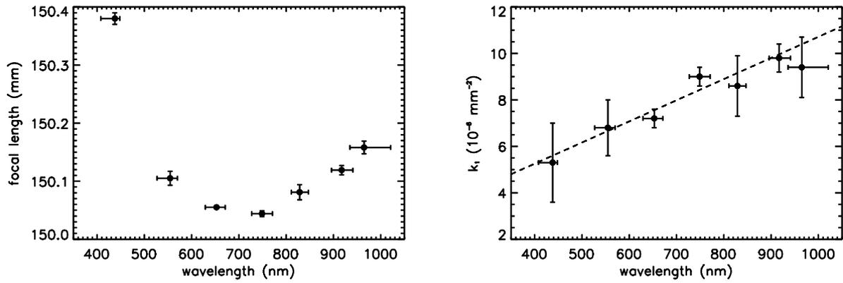
Figure 13. FC2 geometric distortion characteristics. Left: Focal length as a function of wavelength. Right: The radial distortion parameter  $k_1$  depends on wavelength (lateral chromatic aberration). The dashed line is a linear fit to the data.
