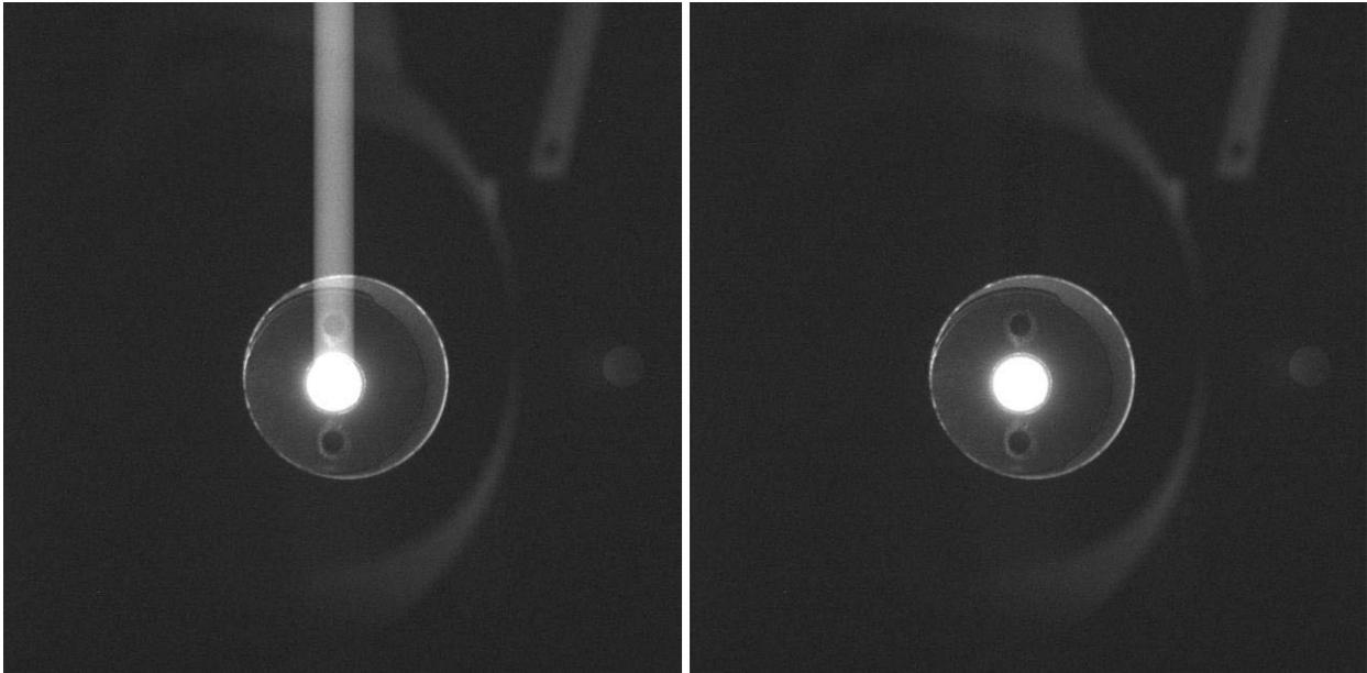
**Figure 5. The de-smear algorithm in action. The FC1 observed an illuminated pinhole through a collimator through F1 (8 Mar 2006). Exposure time was 60 [ms]. Left: original image (average of two). Right: image after de-smearing. The brightness is scaled identically in both, such that black and white are equivalent to  $-5$  DN and 30 DN, respectively. The peak signal in the central spot was 13110 DN. Note that a weak ghost is visible at the right of each image.**
