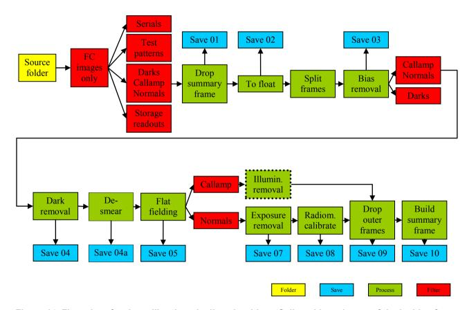
Figure 14. Flow chart for the calibration pipeline algorithm. 'Callamp' is an image of the inside of the camera cover illuminated by the internal calibration lamp (labeled 'flat field' in the PDS image header).
