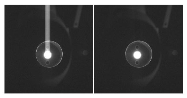
Figure 5. The de-smear algorithm in action. The FC1 observed an illuminated pinhole through a collimator through F1 (8 Mar 2006). Exposure time was 60 [ms]. Left: original image (average of two). Right: image after de-smearing. The brightness is scaled identically in both, such that black and white are equivalent to –5 DN and 30 DN, respectively. The peak signal in the central spot was 13110 DN. Note that a weak ghost is visible at the right of each image.
