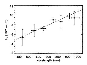
Figure 13. FC2 geometric distortion characteristics. Left: Focal length as a function of wavelength. Right: The radial distortion parameter  $k_1$  depends on wavelength (lateral chromatic aberration). The dashed line is a linear fit to the data.
