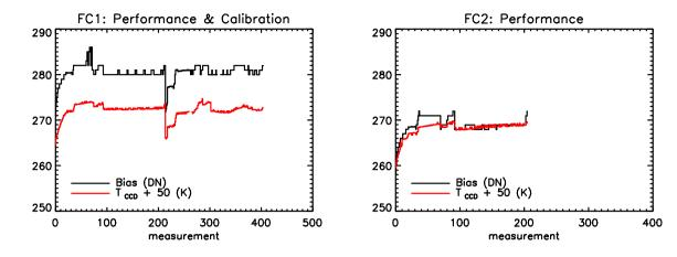
Figure 2. The bias of FC1 images acquired during the ICO *Performance* and *Calibration* blocks compared to the CCD temperature. Left: FC1, right: FC2.
