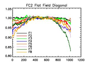
Figure 7. Diagonal profiles through the flat fields in Figure 6, running from pixel [0,0] to [1023,1023]. The profiles have been subjected to a 7-pixel wide median filter.
