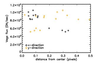
Figure 9. The measured flux of a point source (in this case Vega observed by FC1 through F7) depends strongly on the position of the PSF on the pixel, especially in *x*-direction because of the presence of anti-blooming gates. The *x*-axis denotes the distance of the center of the PSF to the center of a pixel, as determined by a 2D Gaussian fit.
