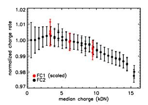
Figure 12. Investigation of CCD linearity. Shown are the mean FC1 and FC2 charge rates in a 100×100 pixel block in the lower left corner as a function of median charge in lab flat field images (FC1: 24 Feb 2006; FC2: 12 Aug 2005). The FC2 charge rate is normalized to that associated with the lowest median charge. The FC1 charge rates were higher, but scaled to match the FC2 series. Some scatter in the data is due to uncertainties in exposure time.
