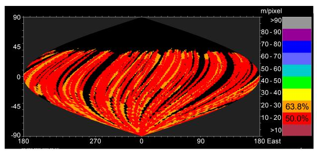
Figure 4-24. Vesta LAMO clear filter image coverage (incidence < 80°).
