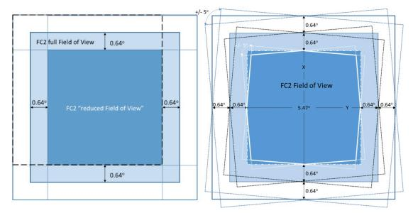
Figure 7–5. Illustration of FC "Reduced FOV".
