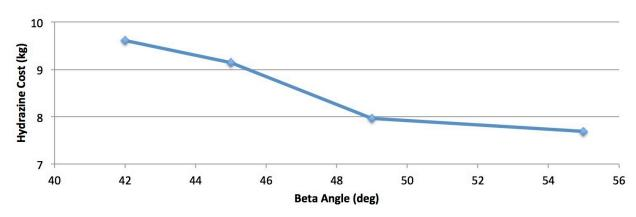
Figure 7-36. Ceres LAMO Hydrazine Cost as a Function of Beta Angle.
