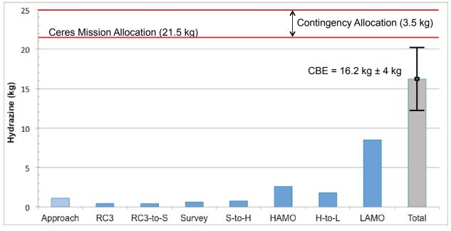
Figure 7-4. Ceres Hydrazine Usage per Sub-phase.
