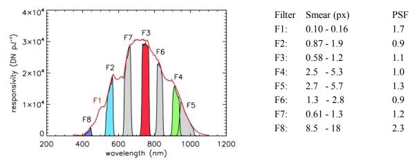
Figure 5–23. FC Filter Wavelength Response and LAMO Pixel Smear and Point Spread Functions.
